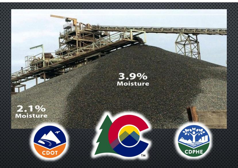
CDPHE wants producers to wash aggregates (reduce air particulates). Some producers require the dust as part of their mix design. The increased moisture content in the aggregate requires more energy to dry and is larger than the initial dust impact. Example of CDPHE vs CDOT and competing goals.
